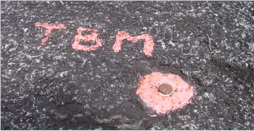
A nail in the middle of a street. TBM – (Temporary Bench Mark). These points are marked for specific projects and generally have good site visibility with long sight lines.
