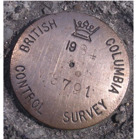
A “Brass Cap” marks this permanent monument installed by the Canadian government in 1984. The dimple that can be seen in the center of the disk marks the specific location that has been measured and recorded.
